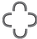
Direction of tubular buttress is easily adjustable
